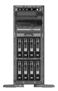
8 SFF hot-plug drive model: Tower - shown without the tower feet.
